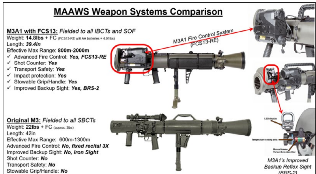
Figure 1 — Comparison of the New M3A1 with FCS13 and Original M3 (Graphic courtesy of author)
