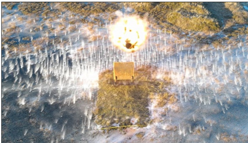
The improved High Explosive (HE) 441E round fires metal spheres at point detonation or airburst with an improved spread pattern than the original HE 441D. The M3A1 adds a fire control unit to the tube that allows the FCS-13 to digitally program when the round explodes on airburst instead of AGs manually rotating the nose cone of the older HE 441D. (Photo courtesy of PEO Soldier)
