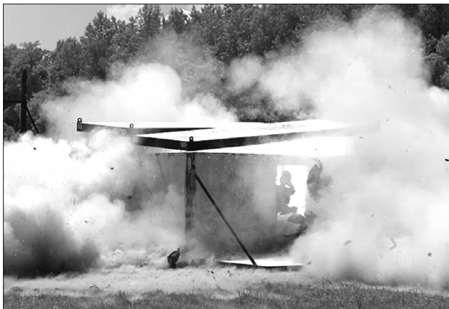
With a thermobaric warhead, the Anti-Structure Munition (ASM 509) can provide effects against multi-story buildings. It also serves well against snipers in built up areas and enemy inside caves. (Photo courtesy of PEO Soldier)
