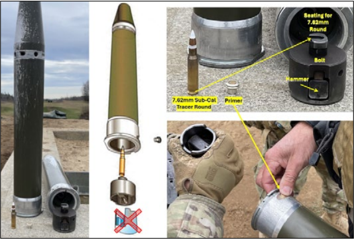
Figure 3 — The 7.62mm Sub-Caliber Adapter (SCA) The SCA is built for a three-part munition system including a unique (low-grain) 7.62mm tracer round, a primer, and a backblast simulator. The backblast simulator (crossed out on below image) is not necessary or valuable for training. It is advised units only use the 7.62mm tracer round and primer. (Graphic courtesy of author)
